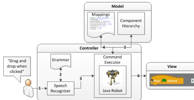
The user states, "Drag and drop when clicked." The speech recognizer identifies the command and checks it against the grammar. If the command exists, the command executor locates the mapping and verifies the state. Finally, the Java Robot performs the corresponding mouse/keyboard action.
